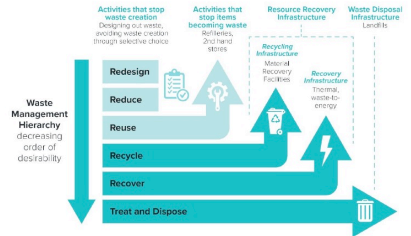
Figure 2: Waste minimisation hierarchy and resource recovery and disposal infrastructure (Te Waihangā, New Zealand Infrastructure Commission, 2020, adapted from s44 Waste Minimisation Act 2008 and Auckland Council, 2018).
